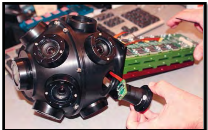
Figure 8 Street View camera system.
